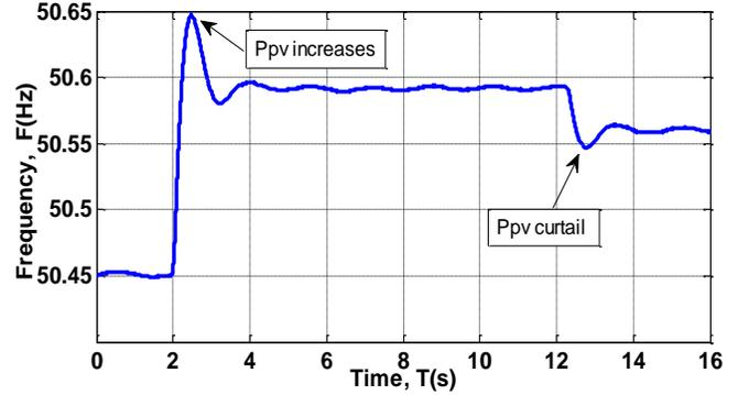
Figure 12. Frequency at the CHIL/PHIL test: applying active power curtailment of the hardware PV inverter.
