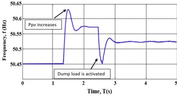
Figure 10. Frequency at CHIL/PHIL test: use of hardware controllable loads.
