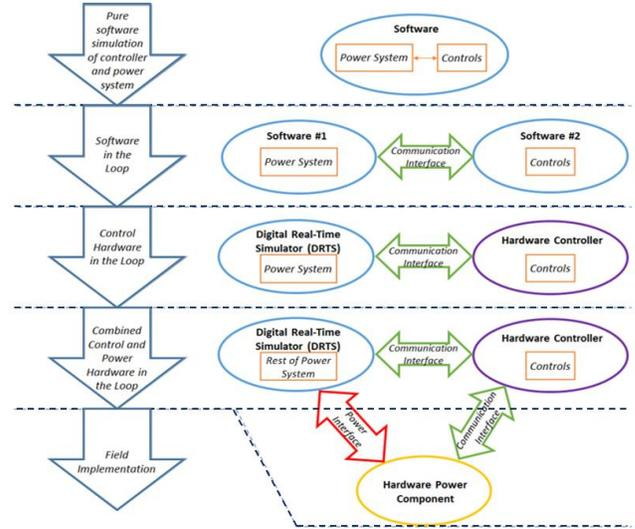
Figure 4. Testing chain for smart grid controllers [29][30].
