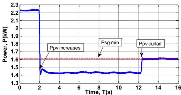
Figure 11. Active power of the DDG at the CHIL/PHIL test: applying active power curtailment of the hardware PV inverter.
