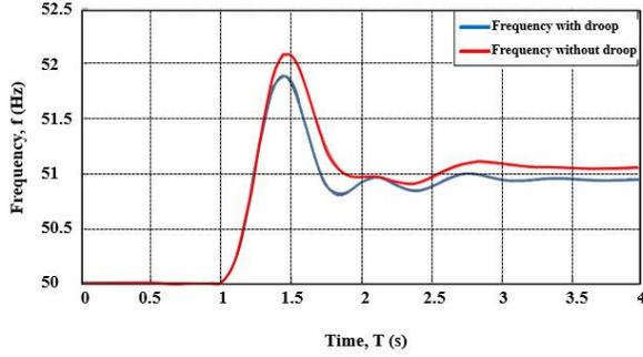
Figure 2. Frequency of a PV-DDG microgrid with and without droop control of the PV inverter.
