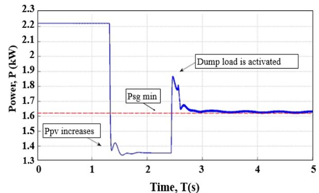
Figure 9. Active power of the DDG at the CHIL/PHIL test: use of hardware controllable loads.
