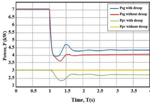
Figure 3. Active power of the DDG and PV inverter with and without droop control of the PV inverter.
