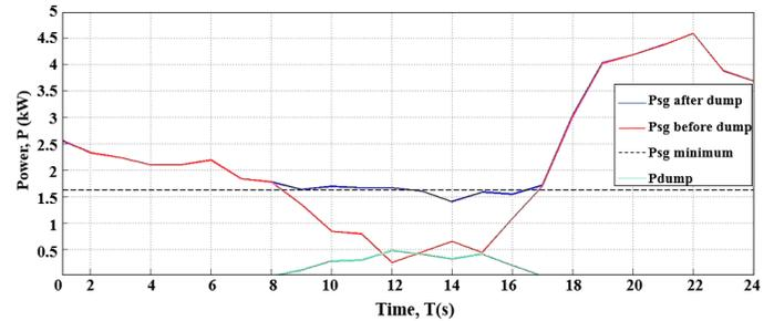
Figure 7. Active power of DDG and hardware controllable loads during daily operation at the CHIL/PHIL test.
