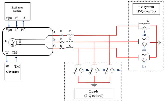
Figure 1. Hybrid DDG-PV microgrid developed in the DRTS software.
