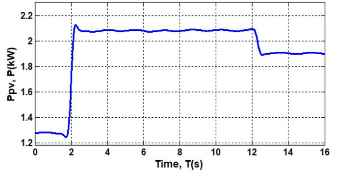
Figure 13. Active power of the hardware PV inverter at the CHIL/PHIL test: irradiation increase and active power curtailment.
