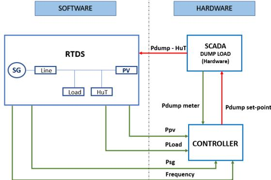
Figure 5. Combined CHIL and PHIL laboratory setup.
