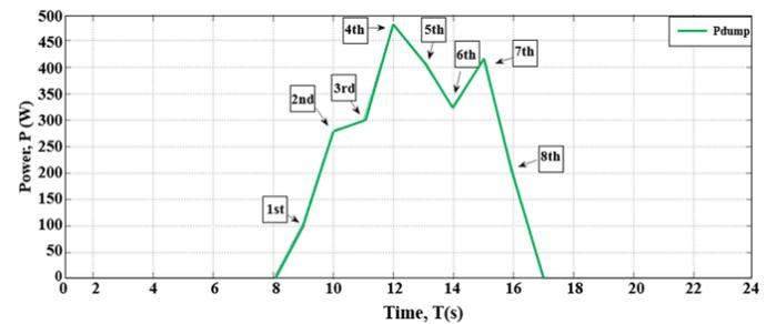
Figure 8. Active power of the hardware controllable loads during daily operation at the CHIL/PHIL test.
