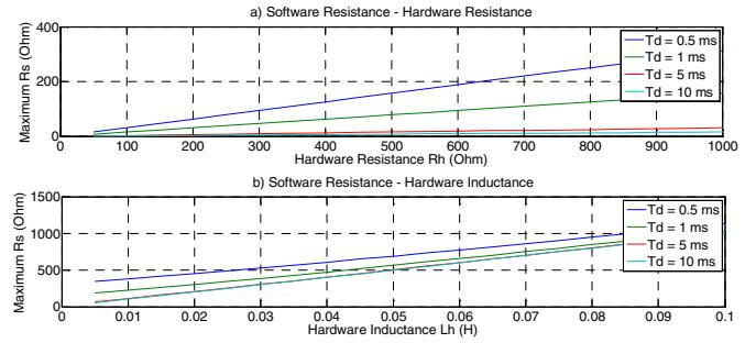
Fig 3. Variation of the software resistance with respect to a) hardware resistance and b) hardware inductance for different time delays
