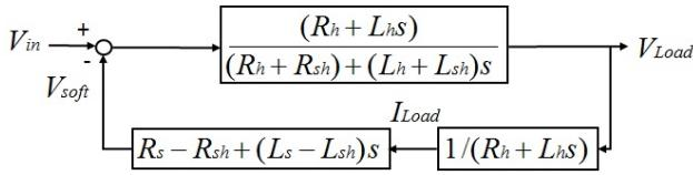
Fig 8. PHIL model with shifting impedance method
