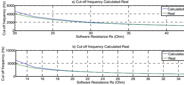
Fig 12. Calculated and real cut-off frequency of the low pass filter-Case 1
