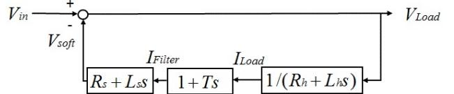
Fig 6. PHIL model with feedback filter
