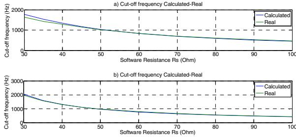
Fig 13. Calculated and real cut-off frequency of the low pass filter-Case 2
