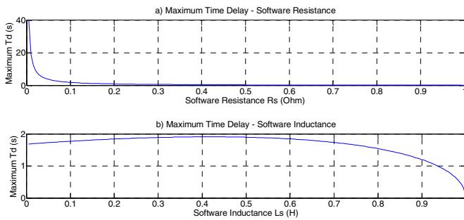
Fig 5. Maximum time delay variation with respect to a) Software resistance  $R_s$  b) Software inductance  $L_s$
