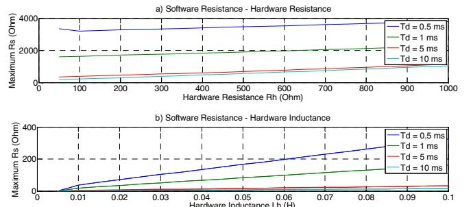
Fig 4. Software resistance variation with respect to a) hardware resistance and b) hardware inductance for different time delays
