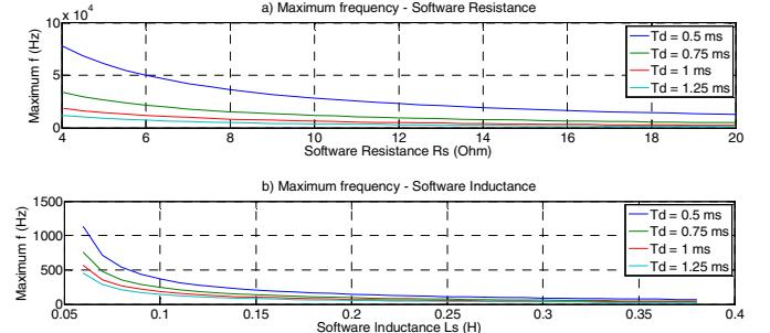
Fig 7. Maximum frequency variation of the low pass filter with respect to the a) software resistance and b) software inductance for different time delays
